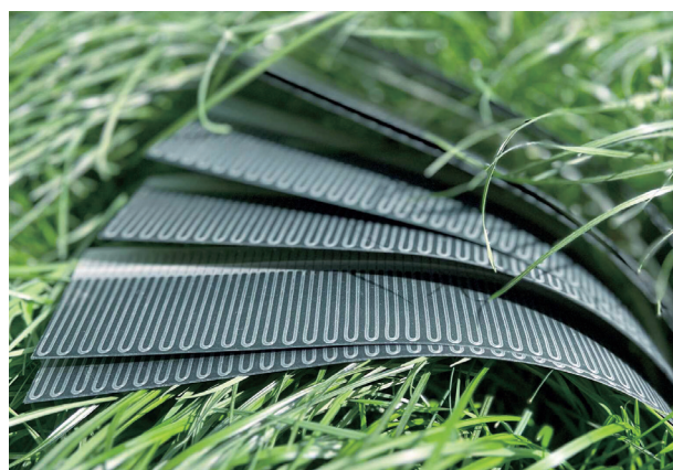
Flexible perovskite/CIGS tandem solar cells developed using the anti-solvent-seeding approach. (Graphic: NIMTE)
