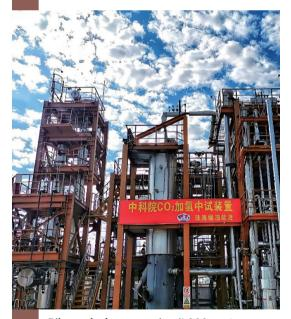
Pilot-scale demonstration (1,000 ton/year) of  $\rm CO_2$  hydrogenation to gasoline, advancing sustainable fuel production by DICP scientists.
