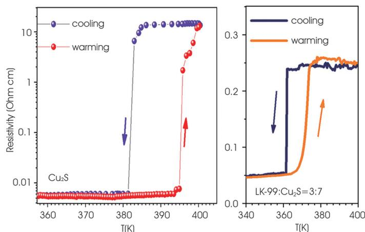
Temperature dependence of resistivity of  $\text{Cu}_2\text{S}$ , LK-99 including  $\text{Cu}_2\text{S}$  (Image by IOP)
