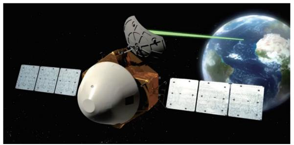
Illustrated on the front of the probe is the lander-rover complex, and in the rear the orbiter. (Image credit: CNSA)
